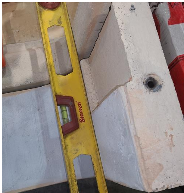
Figure 55: Entrance and exit refractory troughs into the filtering box
