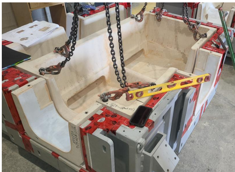
Figure 54: New refractory bowl
