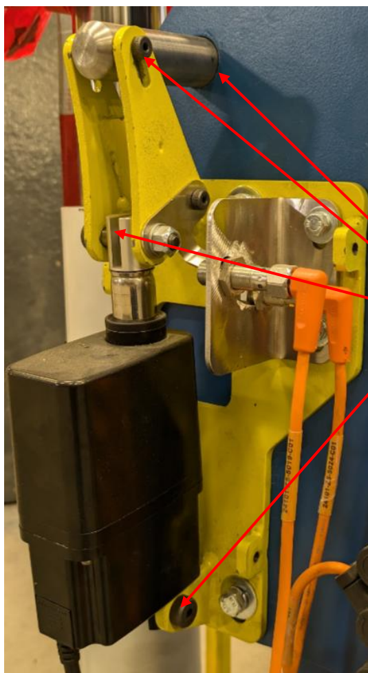
Figure 42 : Greasing points on the locking mechanism
