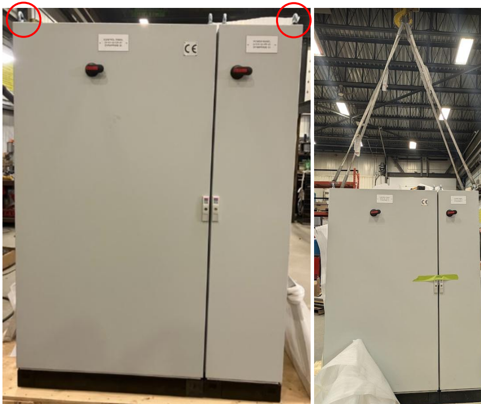
Figure 15 : Identification of the lifting points on the power and control panel
