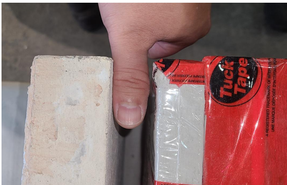
Figure 56: Gap between the refractory bowl and the microporous panels
